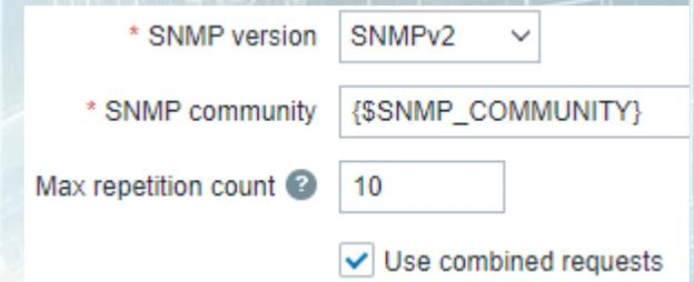
The screenshot shows a configuration panel for SNMP. It includes a dropdown menu for 'SNMP version' set to 'SNMPv2', a text input for 'SNMP community' containing '{\${SNMP\_COMMUNITY}}', a text input for 'Max repetition count' set to '10', and a checked checkbox for 'Use combined requests'.
