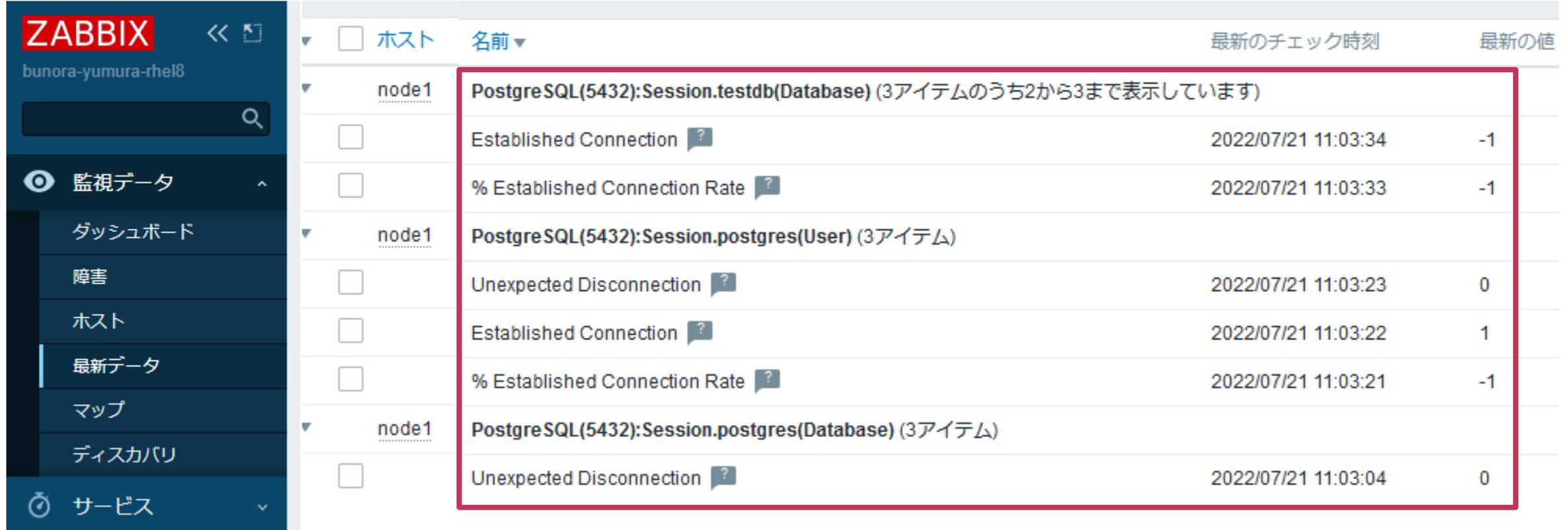
The screenshot displays the Zabbix web interface. On the left is a dark blue sidebar with the 'ZABBIX' logo and navigation menu items: '監視データ', 'ダッシュボード', '障害', 'ホスト', '最新データ', 'マップ', 'ディスカバリ', and 'サービス'. The main content area shows a table of monitoring items for host 'node1'. A red box highlights a section of the table containing PostgreSQL session-related metrics.
