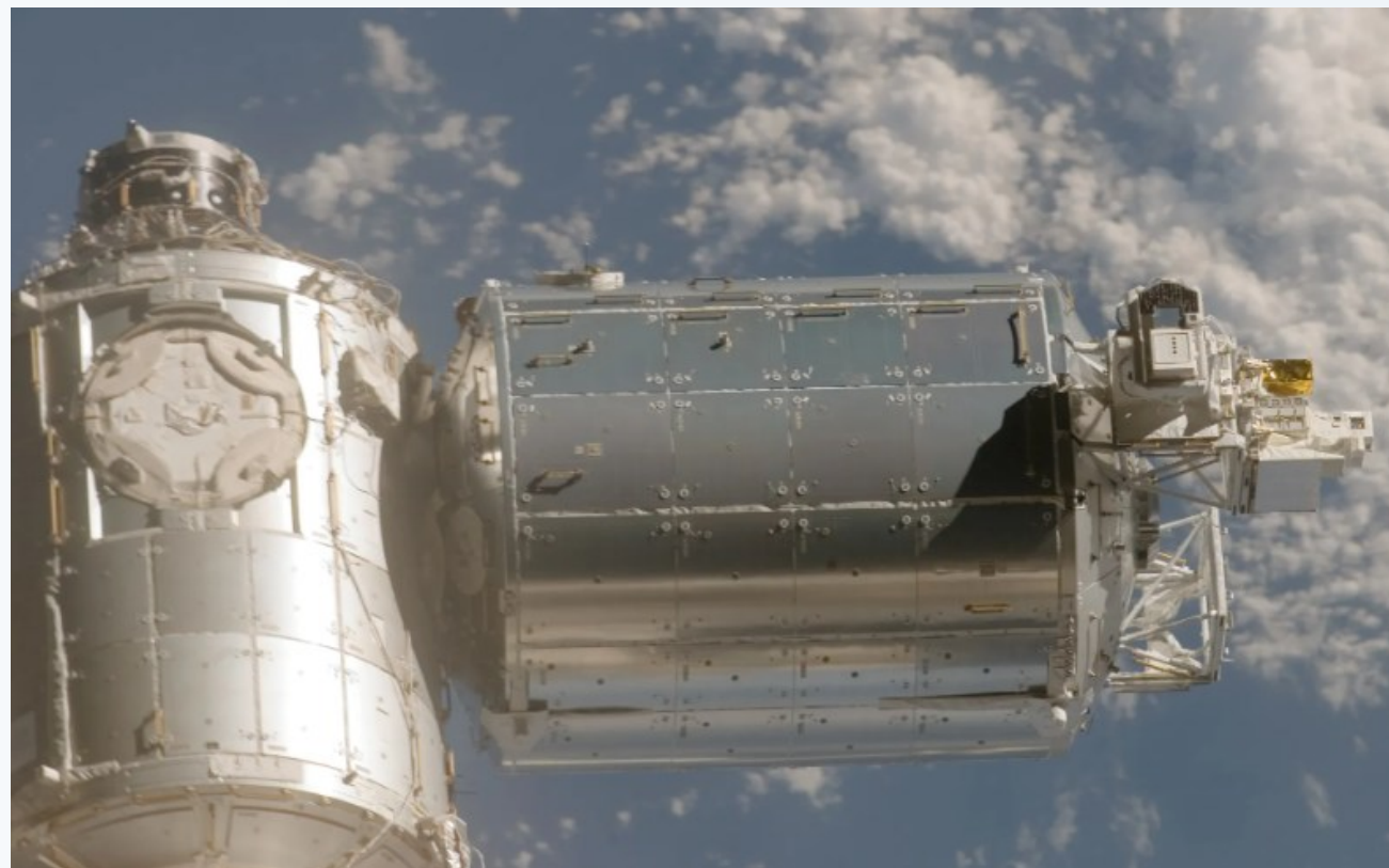
The Columbus laboratory module, from ESA (European Space Agency) attached to the International Space Station's Harmony module by an astronaut aboard space shuttle Atlantis
