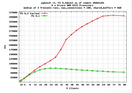
pgbench, scale factor 100, median of 3 30-minute runs, 32-core AMD Opteron 6128 max\_connections = 100, shared\_buffers = 8GB
