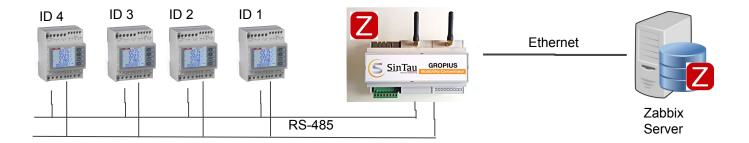
Every multimeters is connected on the same bus and configured with a different ModBus ID
