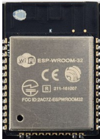
Microcontroller with Wi-Fi and I2C Bus. (Espressif ESP32)
