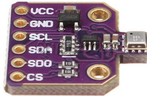
Sensor with I2C Bus (Bosch BME280 / BME680)
